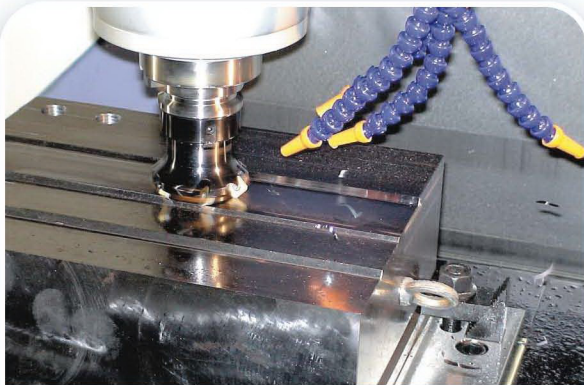
Face milling—S50C Steel
